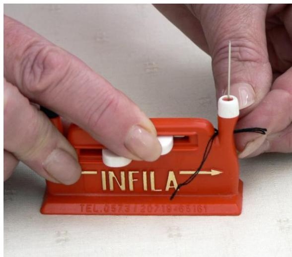
*Fig.3 Automatic needle threader in use*
